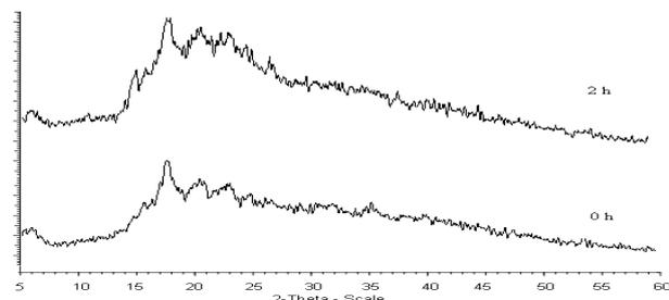
**Figure 6.** X-ray chromatograms of SM 50:50 control and UV-treated for 2 h exposure time
