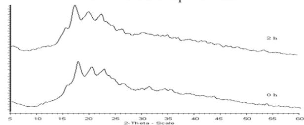
**Figure 7.** X-ray chromatograms of SM 25:75 control and UV-treated for 2 h exposure time
