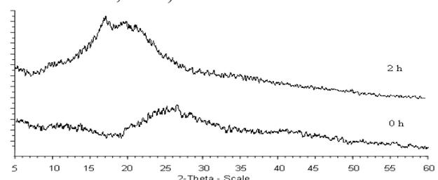
**Figure 3.** X-ray chromatograms of S 100 control and UV-treated for 2 h exposure time
