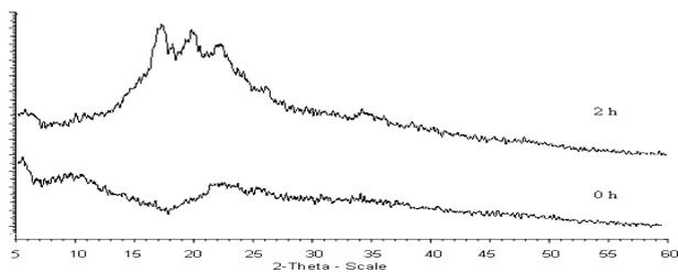
**Figure 4.** X-ray chromatograms of M 100 control and UV-treated for 2 h exposure time
