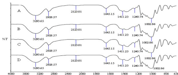
**Figure 8.** FTIR spectra for starch films (control and UV-treated) A) S 100 0h, B) S 100 2 h, C) M 100 0h and D) M 100 2h
