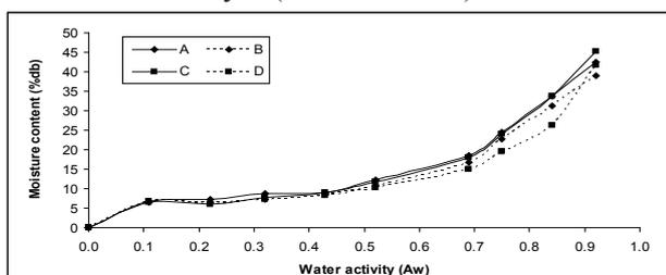
**Figure 1.** Moisture sorption isotherms for starch films, control and UV-treated for 2 h, A) S 100 0h, B) S 100 2h, C) M 100 0h and D) M 100 2h
