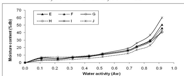
**Figure 2.** Moisture sorption isotherms for starch films control and UV-treated for 2 h, E) SM 75:25 0h, F) SM 75:25 2h, G) SM 50:50 0 h, H) SM 50:50 2h, I) SM 25:75 0h, J) SM 25:75 2 h
