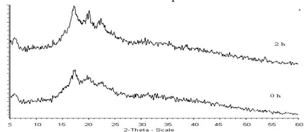
**Figure 5.** X-ray chromatograms of SM 75:25 control and UV-treated for 2 h exposure time
